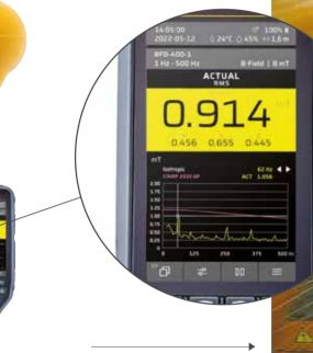
High intensity pulsed magnetic fields occur very close to welding equipment. These fields can be precisely detected and evaluated with the aid of the Narda H field
