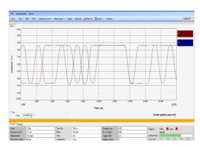
IQ-Data-View for detailed analysis of digital modulated signals (Screen NRA Scope Demo Software)
