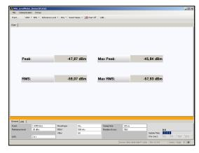
True RMS analysis by selecting Fcent and RBW (Screen NRA Level Meter Demo Software)
