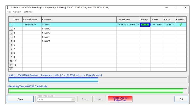
The 8063SW02 software is a control program fully integrated into the system that enables changing setting, querying and monitoring all the installed units.
