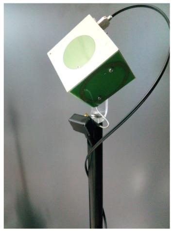
The electromagnetic field analyzer
