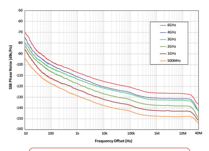
FIGURE 3: Phase Noise Performance (typical), Pour Setting: +10dBm
