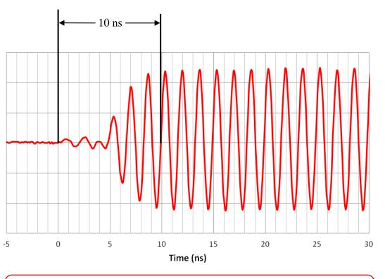
Figure 20: External Pulse Modulation Rise Time (seconds)
