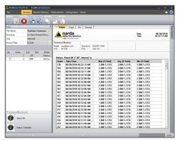
The contents of the data recorder can be read out and displayed very conveniently using the RadMan 2-TS PC software.
