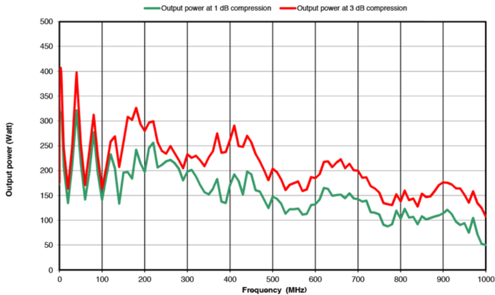
DT150 POWER AMPLIFIER 150W / 10 kHz - 1000 MHz
