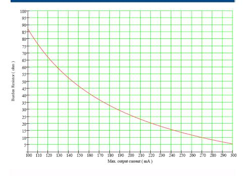
To maintain safe start-up  $\mathbf{R}_{\mathrm{M}}$  must not exceed 20  $\Omega$  during fault condition.
