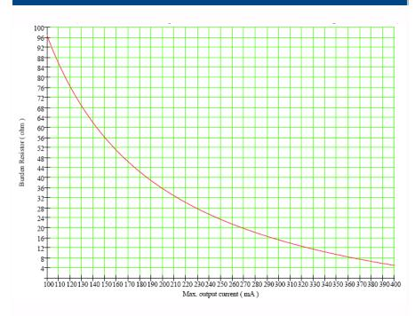
To maintain safe start-up  $\mathbf{R}_{\scriptscriptstyle M}$  must not exceed 30  $\Omega$  during fault condition.
