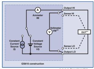
\*1: DUT: Device Under the Test
