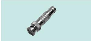
Used to connect an oscilloscope having a 1 MΩ input to a probe with a 50-ohm output. Frequency range: DC-500 MHz. Allowable power: 0.5 W.
