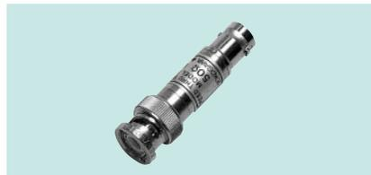
Used to connect an oscilloscope having a 1 MΩ input to a probe with a 50 Ω output. It is required when using the 701920 and 701922 probes with the DL1600 series.
