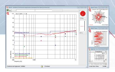
In the commercial radiated emissions test the signal level vs. turntable rotation and antenna mast height are plotted at each final test frequency, along with the original swept frequency data and tables of results for each detector used.
