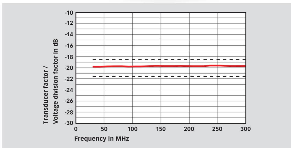
Typical decoupling of CM disturbance (RF Out port/AE)
