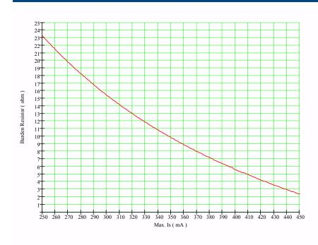
To maintain safe start-up  $\mathbf{R}_{_{\mathrm{M}}}$  must not exceed 2.5  $\Omega$  during fault condition.
