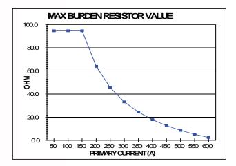
To maintain safe start-up  $\mathbf{R}_{\scriptscriptstyle{\mathrm{M}}}$  must not exceed 2.5  $\Omega$  during fault condition.
