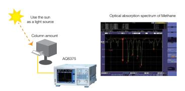
Figure 4 – Measurement setup to detect a specific gas in the air, e.g. Methane ( $\mathrm{CH_4}$ )
