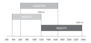
The AQ6375 is the first bench-top optical spectrum analyzer covering the long wavelengths over 2  $\mu$ m. It is designed for researchers and engineers who have been struggling with inadequate test equipment to measure in these long wavelength ranges. The AQ6375 achieves high speed measurements with high accuracy, resolution and sensitivity, even while providing full analysis features. Troublesome calibration steps and the development of external analysis software is no longer required.
