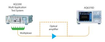
Figure 1 – The typical experimental setup for optical amplifier testing.
