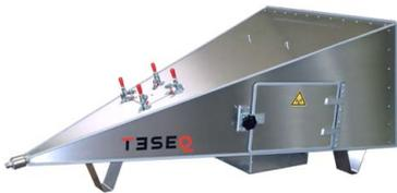
A GTEM (Gigahertz Transverse Electro Magnetic) cell is a test site for efficiently performing both radiated immunity and emissions testing in a single, controllable and shielded environment. Compared to other test sites, GTEM testing is faster with high accuracy and excellent reproducibility.
