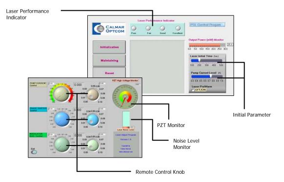
Figure 13 - Remote Control Interface
