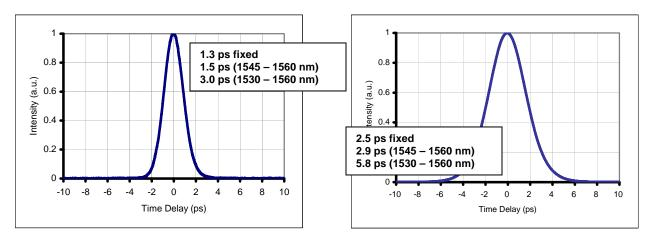
Figure 2 - Pulse Width FWHM of 1.3 ps (Calmar PSL-10-1)
