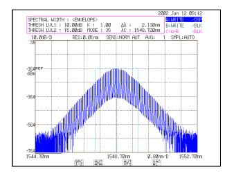
Figure 4 – Spectral Width of 2.1 nm (Calmar PSL-10-1)
