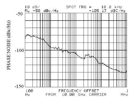
Figure 8 - Timing jitter of 45 fs
