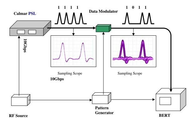
Figure 9 – Test Set-up for BER Measurement
