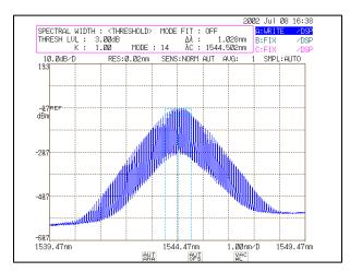
Figure 5 – Spectral Width of 1.0 nm (Calmar PSL-10-2)
